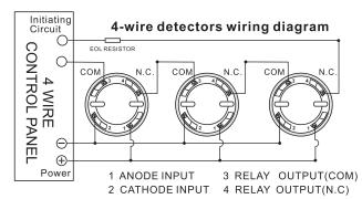
Base terminals "1" and "2" for DC power input, non-polarized. "4" for DC power anode or cathode output."3" for relay output COM. "4" for relay output N.C. or N.O..
