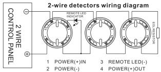
Base terminals "1" and "2" for DC power input, non-polarized. "4" for DC power anode or cathode output. "3" for remote indicator cathode. When remote indicator is used, "1" must be connected with the positive power input line.
