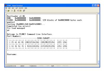
Figure 5-1: IGSW-24040T Managed Switch Console Login Screen
