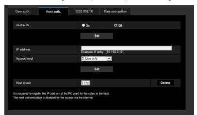
The restriction settings of PCs (IP address) from accessing the camera can be configured on this page.
