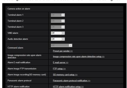
The settings related to the camera action on alarm can be configured in this section.
