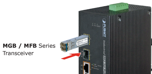
Figure 2-3: Plug-in the SFP transceiver
