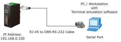
A terminal program is required to make the software connection to the IGS Managed Industrial Switch. Windows' **Hyper Terminal** program may be a good choice. The Hyper Terminal can be accessed from the Start menu.
