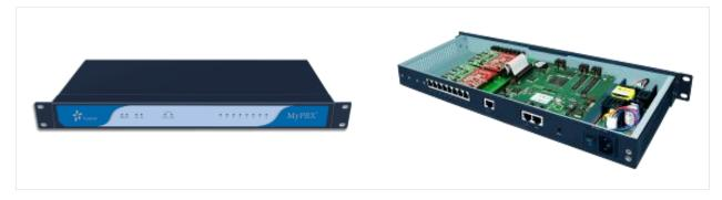
Size: 440x175x45mm (1U Rack-Mount) Weight: 2500g Power Supply: 90V~264V, 50~60Hz 1.5A MAX
