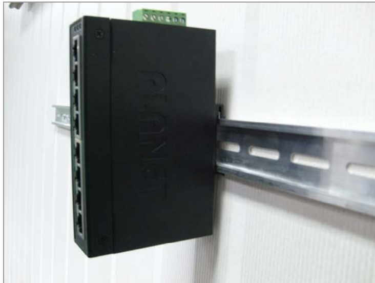
Figure 2-10 Industrial Equipment installed in DIN-Rail mount.
