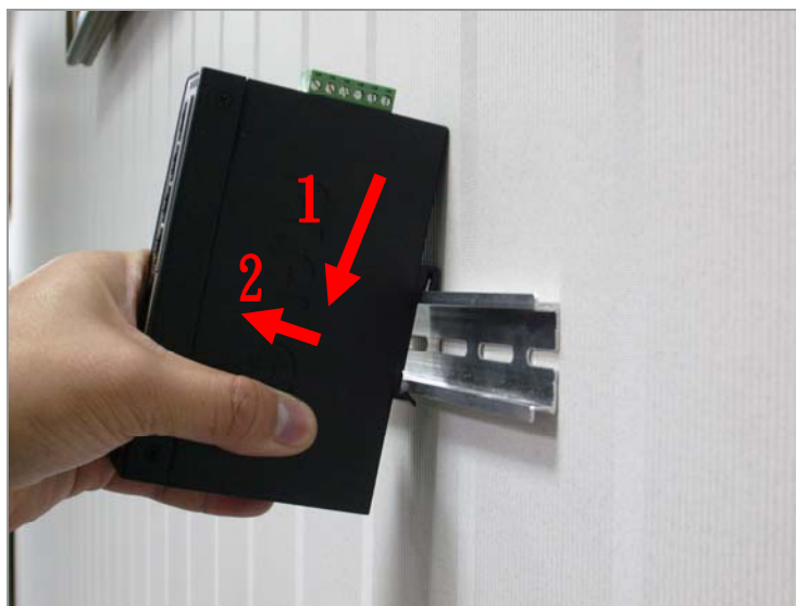
Figure 2-11 Remove Industrial Equipment in DIN-Rail mount.
