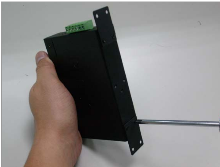
Figure 2-12 Attach brackets to the Industrial Equipment.
