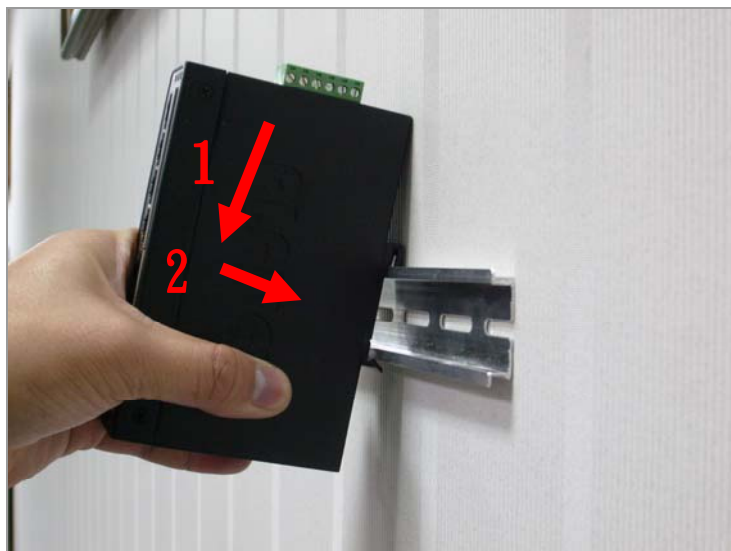
Figure 2-9 Install Industrial Equipment in DIN-Rail mount.
