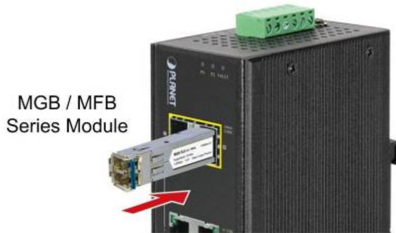
Figure 2-5: Plug-in the SFP Transceiver
