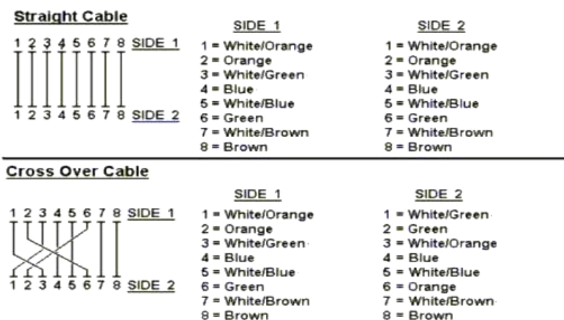
Figure A-1: Straight-Through and Crossover Cable
