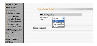
WDS security setting provides three encryption modes: WEP encryption, TKIP encryption and AES encryption.
