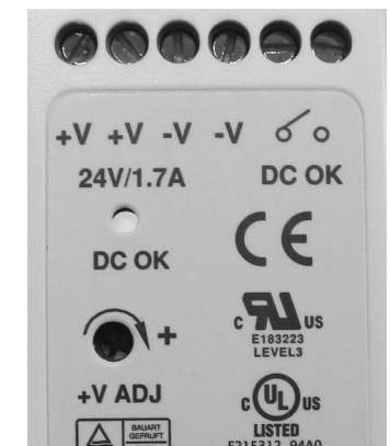
Figure 2. "DC OK" LED of DC Single Output Industrial DIN Rail Power Supply units.
