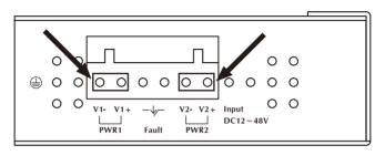
2. Tighten the wire-clamp screws for preventing the wires from loosing.
