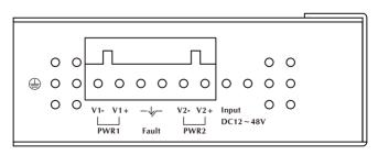
Figure 2-6 Industrial Fast Ethernet Switch upper Panel.
