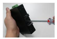
**Step 2:** Lightly press the button of DIN-Rail into the track.
