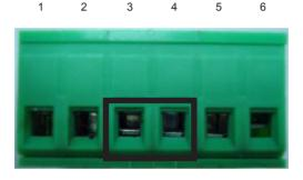
Insert the wires into the fault alarm contacts
